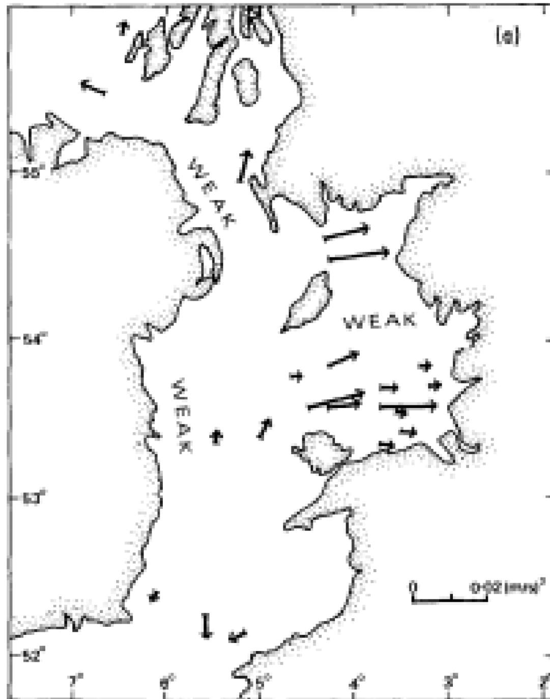
Figure 22 Net directions and relative magnitudes of sand transport in the Irish Sea (Kenyon and Cooper, 2005)
